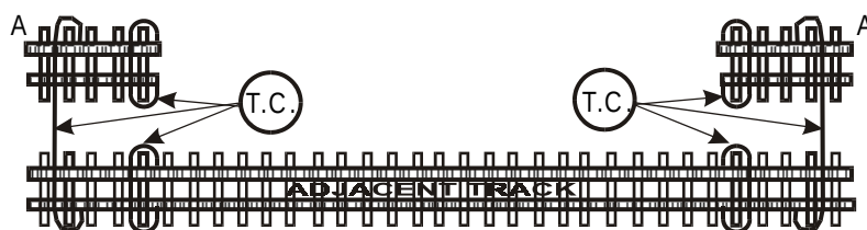
4) REMOVING BOTH THE RAILS SIMULTANEOUSLY OF ONE LINE (ALTERNATIVE TO NO. 2 ABOVE)
