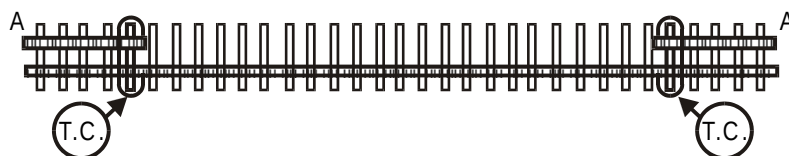
1) REMOVING OF ONE RAIL (BOTH THE RAILS INSULATED FOR TRACK CIRCUITING)
